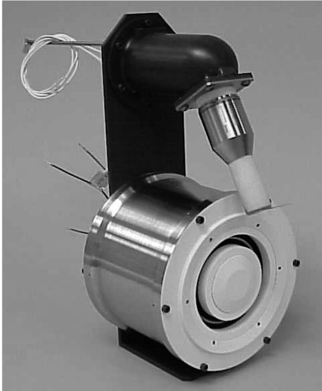
Fig. 1 Photograph of circular BHT-600 Hall thruster used in this study.
