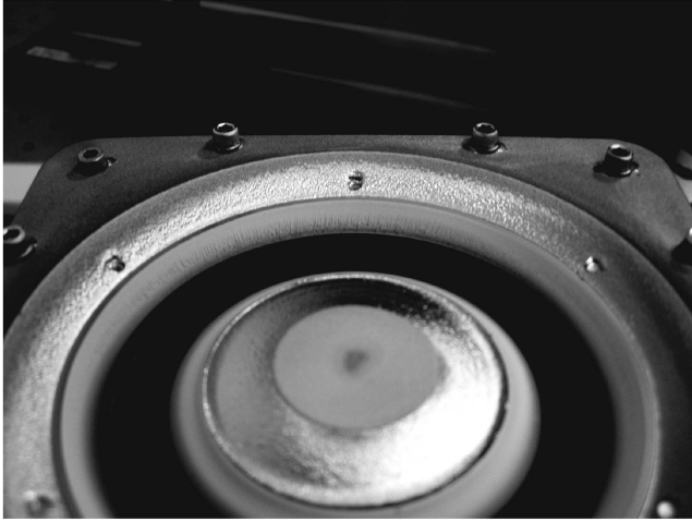
Fig. 9 Front surface erosion of a rectangular BHT-600 thruster following extended operation. Note the exposed metal at the thruster center where the protective alumina covering has been eroded.
